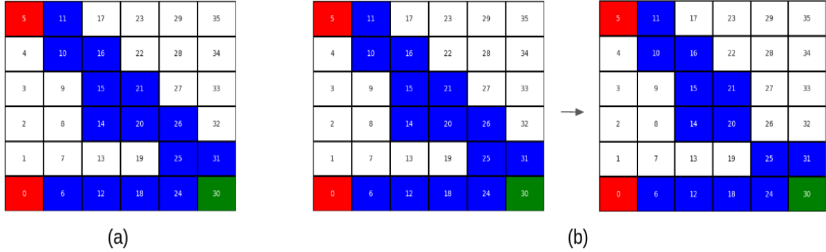
Figure 6: Illegal actions. (a) Removing voided (white), loaded (green), bounded (red) cells. (b) Action results in non-singular body such as removing cell 26 for given example.
